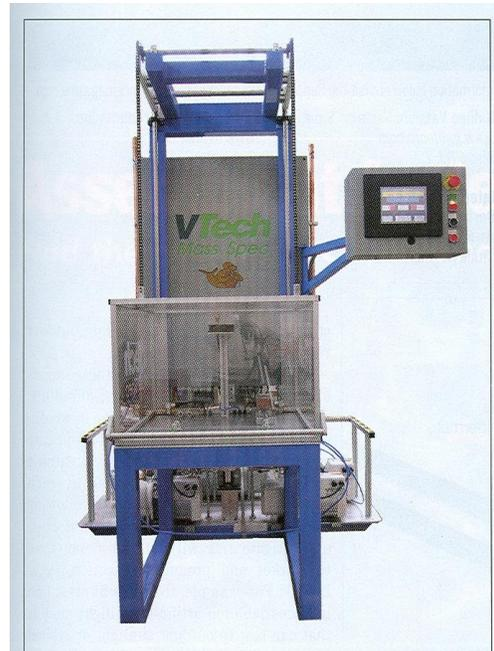
*The VTech (Alpharetta, Georgia, U.S.) MasSpec is an automatic helium leak detector for testing refrigeration components and complete refrigeration units, even in the presence of polyurethane foam. It detects helium leaks as small as 0.1 oz of R-134a per year. It requires just 10% helium concen-*
