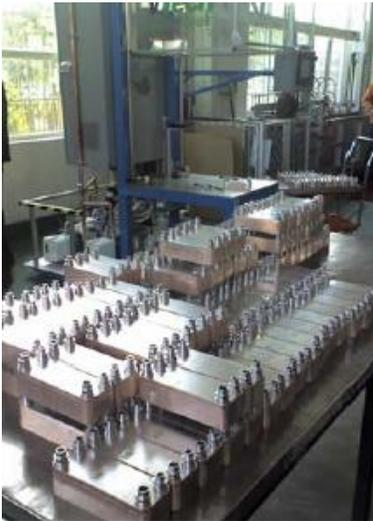
Kaori is currently using the VTech MasSpec for the integral leak detection of their brazed plate heat exchangers. The quality of the leak testing is certified by a calibrated leak and the testing results are recorded to a database for data mining and/or print out of testing certificates.
