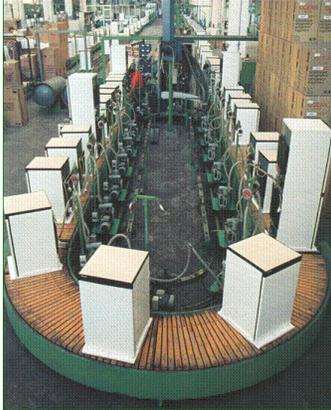
Most manufacturers' evacuation realization consists of a moving production line or carousel where each refrigeration circuit or other product is attached to a single smaller rotary pump (10-20 m<sup>3</sup>/h). This method eliminates every one of the disadvantages of the manifold system while adding additional benefits.
