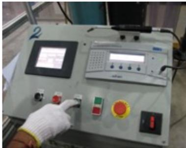
**VTech 75 Multifunction Leak Detection System**
