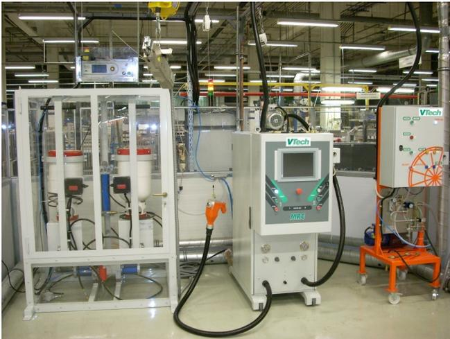
HC Installation including Supply, Charging and Purging
